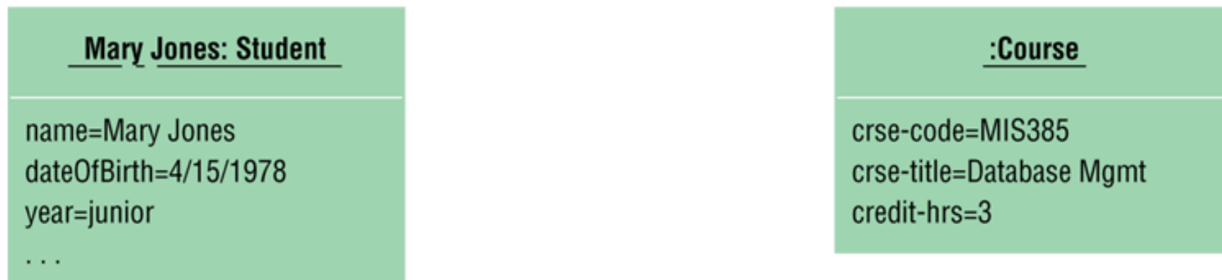
Figure A.3b UML Class and Object Diagrams — Object Diagram with Two Instances
